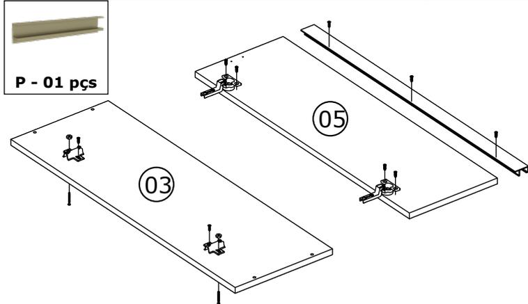
1 - FIXAR OS CALÇOS "H" COM PARAFUSO "E" (M4x25), A PORCA "F" (M4) E O PARAFUSO "C" (3,5x14). EM SEGUIDA FIXAR A DOBRADIÇA "G" E O PUXADOR "P" COM PARAFUSO "C" (3,5x14).
